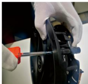
2. Rotate the mounting bracket to the left.
