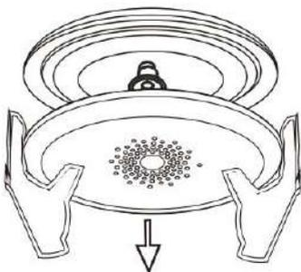
Step 3: Press the open hole in advance, install the product to the ceiling, and lock the screws.
