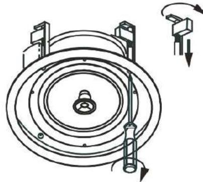
Step 4: After the product is fixed, reload the mesh mask.
